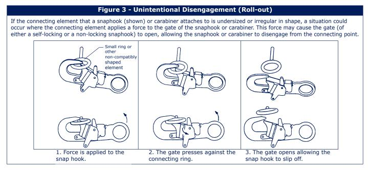
**2.3 MAKING CONNECTIONS:** Only use self-locking snap hooks and carabiners with this equipment. Only use connectors that are suitable to each application. Ensure all connections are compatible in size, shape and strength. Do not use equipment that is not compatible. Ensure all connections are fully closed and locked .
