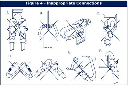
**WARNING:** Do not alter or intentionally misuse this equipment. Consult DBI-SALA when using this equipment in combination with components or subsystems other than those described in this manual. Some subsystem and component combinations may interfere with the operation of this equipment. Use caution when using this equipment around moving machinery and electrical hazards. Do not loop the lanyard around small structural members.
