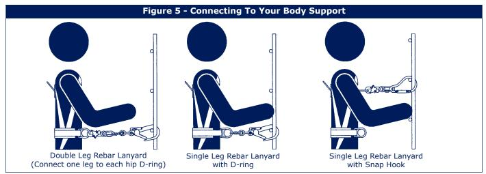
**Single Leg Rebar Lanyards with Snap Hook:** Connect the snap hook to the front D-ring on your cross-over style full body harness. If using this rebar lanyard with a waist belt, slide the waist belt D-ring to your front and connect the snap hook.
