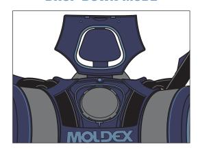
Open valve cover by pulling up on the latch. Pull the straps out from underneath the tabs of the strap channel. Close and snap shut the valve cover.
