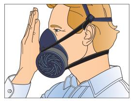
**Positive Pressure Seal Check: Cover** the exhalation valve vent without pressing too hard against face, and exhale gently to create a slight positive pressure. If air leakage is detected, re-adjust the position of the facepiece and the tension of both headstraps and repeat the seal check until leakage is eliminated.
