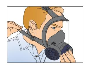
Push facepiece onto face and chin with one hand and position for most comfortable and secure seal while pulling and tightening neck tab of harness with other hand. Repeat for other neck tab. For easiest, most secure and best fit, always adjust neck harness tabs first before tightening top harness tabs.
