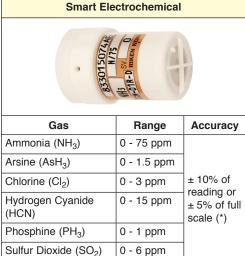
Monitor a wide variety of toxic gases. Smart plug and play sensors are auto recognized and can be remotely calibrated.
